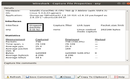
Gambar 1. Tampilan capture wireshark mencari nilai packet loss
